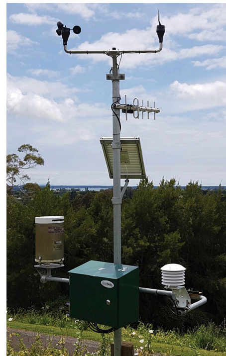
Weather station data is collected and fed into the online Psa Risk Model.
