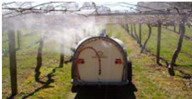
Airblast sprayer fitted with conventional (left hand side) and air inclusion (right hand side) nozzles.
